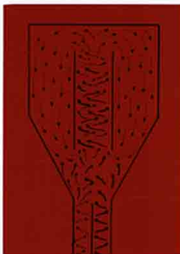
Speed difference between augers creates three-way mixing action.
