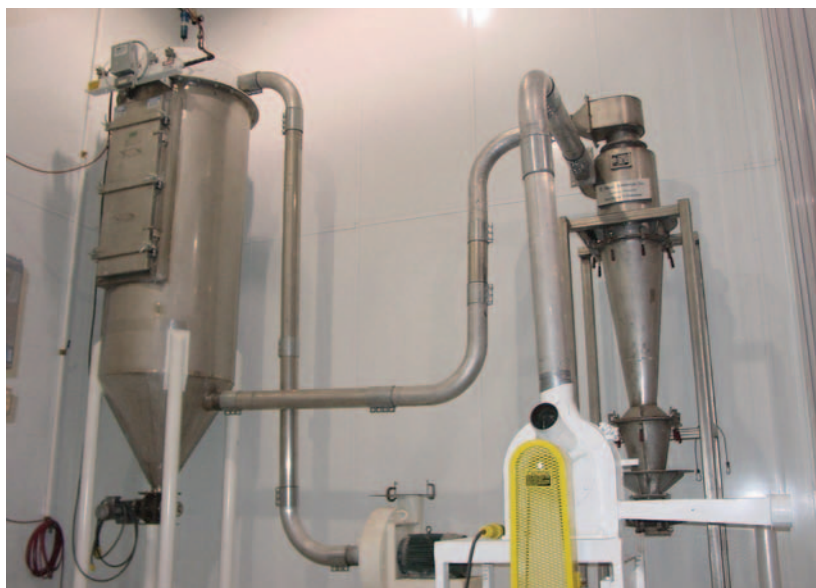
In another area of the test lab, the supplier conducts equipment tests for another customer using a classifying mill (front right), a cyclone separator (back right), and a dust collector (left).
